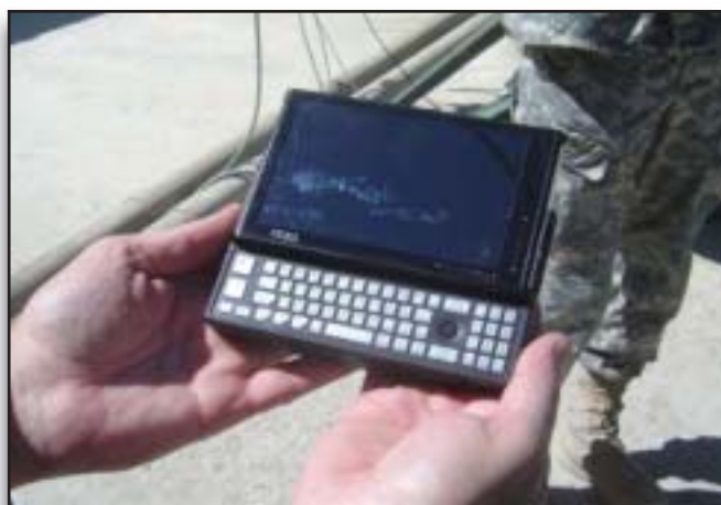
Device shown is a small, handheld computer made by OQO. It is a commercial, off-the-shelf computer provided to communicate with the ODA terminals. Photo by Maj. Thomas Follmer.
